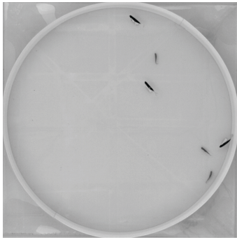
Fig. 8. The view of the experimental setup (described in Fig. 2 with a circular arena (diameter of 580 mm) made of plexiglas. We used three fish-robots and three zebrafish.
