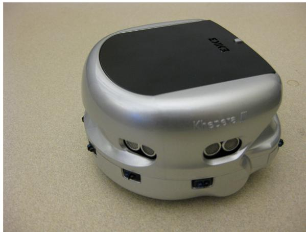
Figure 18: The Khepera III Robot
