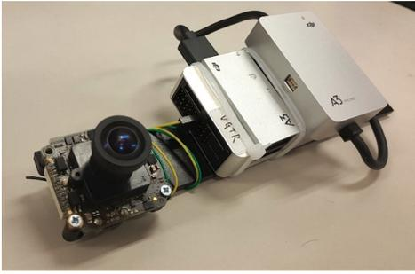
Fig. 12. The device we used for the indoor experiment. It contains one global shutter camera (MatrixVision mvBlueFOX-MLC200w) with  $752 \times 480$  resolution. We use the built-in IMU (ADXL278 and ADXRS290, 400Hz) from the DJI A3 flight controller.
