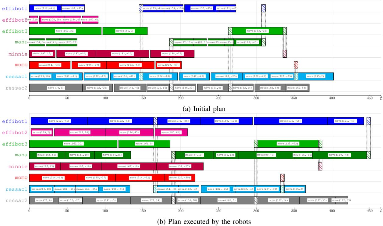
Fig. 6: Temporal representation of plans (x-axis in seconds). Each line represents the plan of one robot. Communications between two robots are represented by the dashed vertical bars. Observation actions are not visible as their duration is null.
