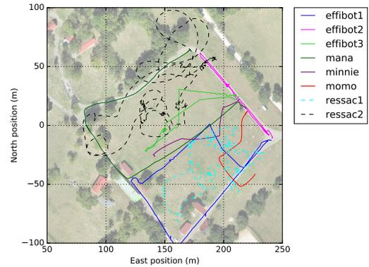
Fig. 5: Trajectory performed by the robots during the mission with only delays (no online repair needed). *ressacs* are aerial robots as shown in Fig. 1, *effibots* are ground robots that can evolve on paved roads, other robots are all-terrain ground robots as shown in Fig. 1.
