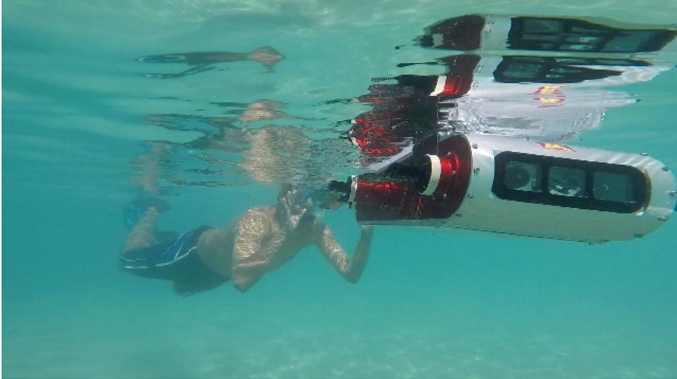
Figure 1: An example of a diver interacting with the Aqua AUV, instructing the robot with free-form hand gestures.
