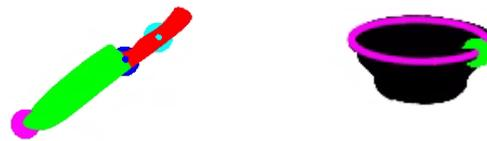
Fig. 4: Left: Tool’s outputs: heel point (blue), grasp point (cyan), tip point (magenta); Right: target object’s outputs: aperture superellipse (magenta); edge point (cyan).
