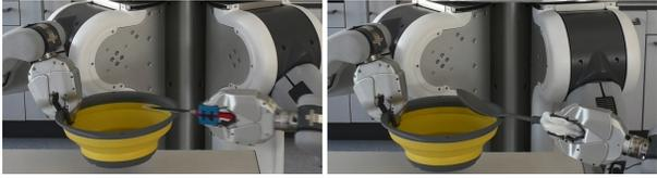
Fig. 7: PR2 scraping across the bowl edge with a small knife (left) and large serving spoon (right). Please see the attached video for further examples on the PR2 robot.
