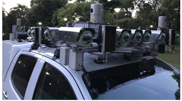
Fig. 2. A close-up of the sensor suite on the AutoVision vehicle platform.
