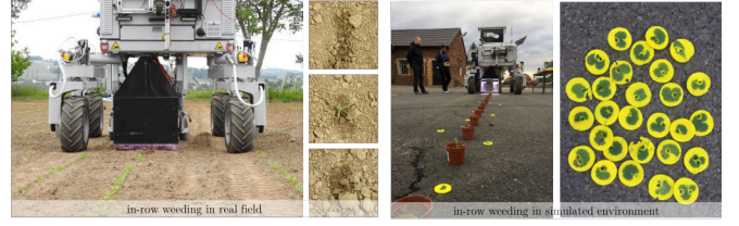
Fig. 6: Left: an in-row mechanical weeding and spraying test is conducted in the real-world field in Ancona, IT. The weeds after spraying can be seen in the picture, and the mechanical treatment results are not visible on the ground. Right: the performance of in-row mechanical weeding is presented in a simulated test environment in Bonn, GE. The faked targets made of leaves attached to modeling clay is utilized to visualize the execution results.
