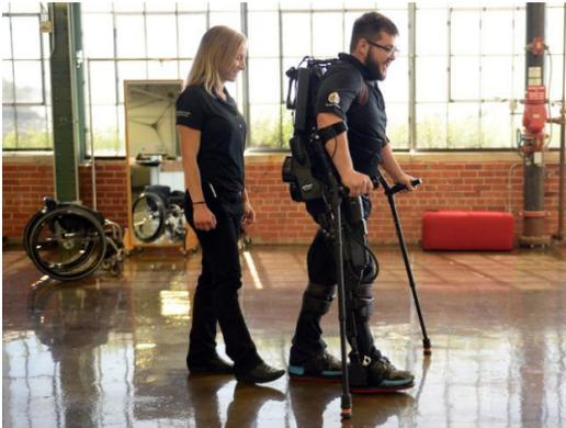
Fig. 3. Ekso Bionics exoskeleton, EksoGT<sup>TM</sup>, used for data collection. We use two sets of its sensors in this study: hip and knee encoders to generate kinematics-based dynamical models using the NCD algorithm, and foot-mounted pressure sensors at the heel and toe to validate our models against ground-contact events after partitioning.
