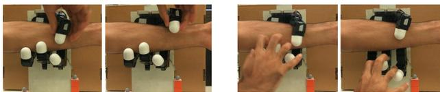
Fig. 12: The compliance of the Allegro hand during the massage. Since the fingers are controlled in the torque mode, they remain compliant to interaction with the human receiving the massage. This behavior guarantees the safety of the interaction.
