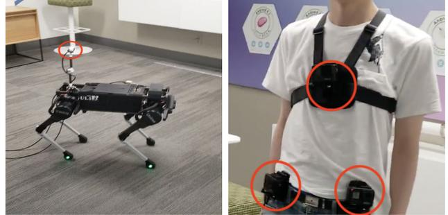
Fig. 1. We develop a learning framework that trains a visual navigation policy for a legged robot (Left) from human demonstrations mounted with three cameras (Right). The red circles indicate cameras.
