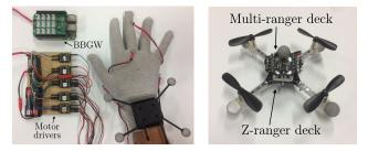
Fig. 3: Wearable interface with hardware control device (left) and CrazyFlie 2.1 equipped with proximity sensors (right).
