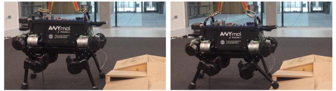
Fig. 10: The mockup terrain with random inclinations
