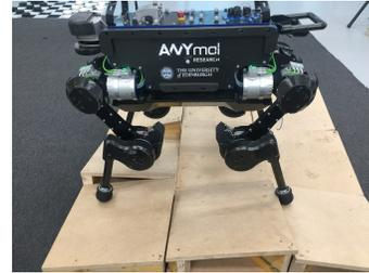
Fig. 1: ANYmal robot walking over an uneven terrain
