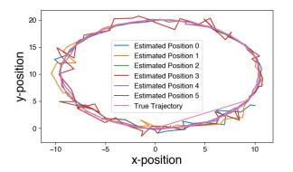
Fig. 3: Comparison of the target agent's true trajectory and its estimate by each robot in a tracking team of six, labeled 0-5.
