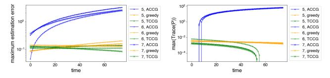
Fig. 6: A comparison of *maximum estimation error* and *maximum*  $Tr(\mathbf{P})$  between the three different strategies for simulations in which only a single node experienced sensor deterioration. Here, **TCCG** performs best for all simulated team sizes.
