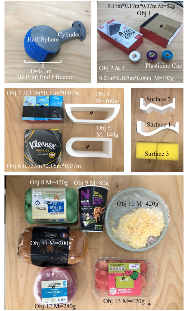
Fig. 6: End-effector, target objects, and support surfaces. Top left: 3D Printed end-effector with blue bandage to increase friction. Top right: object 1, 2, 3 with varying size and mass; plasticine cups for changing the objects’ mass and as disturbances. Middle left: object 4, 5, 6, 7 as target object. Middle right: support surfaces 1 & 2 with curve shape and zigzag shape respectively; sponges as deformable support Surface 3. Bottom: a box of eggs (Obj 8), a cup (Obj 9), a filled bowl (Obj 10), a bag of bread (Obj 11), a cylindric-shaped ham (Obj 12), a full plastic container (Obj 13).
