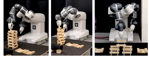
(b) ABB YuMi builds Keva structures using a STAMP policy: 12-level tower (left), twisted 12-level tower (center), and 3-towers (right).
