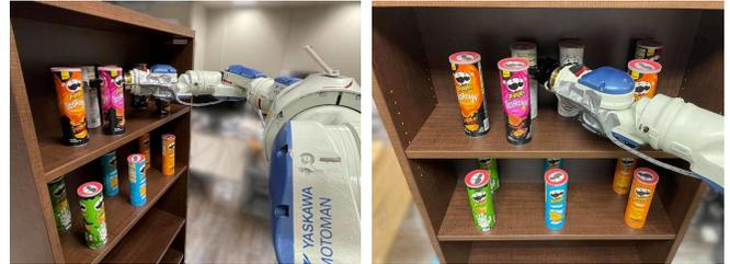
Fig. 1. (left) An example rearrangement problem in a confined space. (right) The problem is challenging even with a few objects as the swept volume of the arm’s motion can easily lead to collisions.
