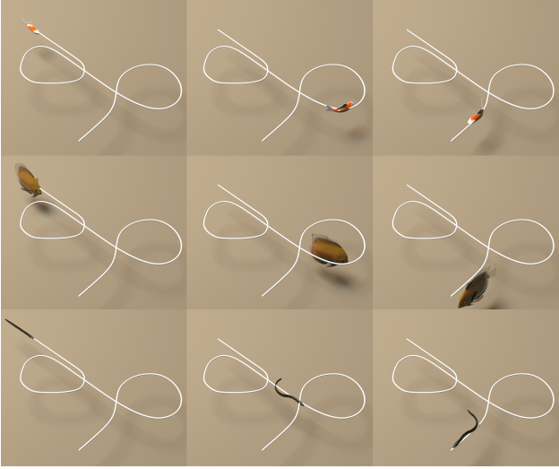
Fig. 6. Different types of robot fishes trained using local policy learning for arbitrary path following. Top: koi robot fish; middle: flatfish robot fish with a different skeleton topology (with branching during modeling); bottom: eel robot fish with a long concatenated skeleton.
