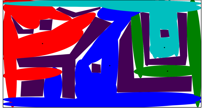
Fig. 1. Example ellipsoid decomposition of the “Jagged” environment and region assignment for team of tracking agents, with obstacles shown in purple and region assignments shown in red, green, blue, and cyan.
