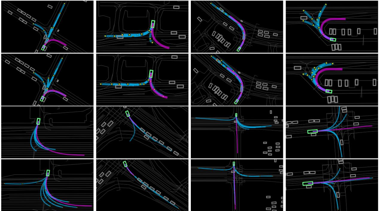
Fig. 3. Samples from WOMB dataset. The agent to be predicted is shown in cyan with its ground truth trajectory shown in magenta. 6 predicted trajectories are shown in blue with yellow stars annotating the keyframes. We compare KEMP-I-LSTM with Multipath. 1st and 3rd rows: Multipath; 2nd and 4th rows: KEMP-I-LSTM.
