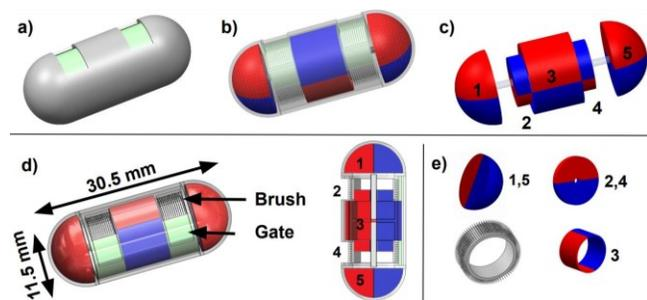
Figure 1. 3D model of the endoscopic capsule: a) external view with closed gates; b) the capsule wall is removed to see the internal components; c) internal magnets arranged inside the capsule; d) the gates (in green), when opened, exposes the brushes (in grey) to the external environment; e) 3D CAD of the five internal magnets and one of the two brushes.
