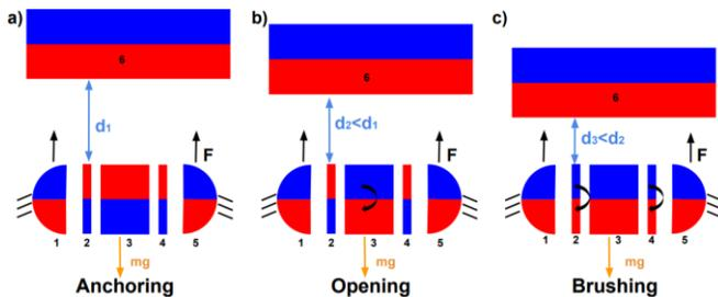
Figure 3. Diagram of the three operational phases and the polarization of the IPMs: a) capsule configuration in rest position, the EPM generate an attraction force on the IPMs; b) the EPM moves forward triggering the IPM<sub>3</sub> rotation (first unstable equilibrium point); c) the EPM moves closer, enabling the rotation of IPM<sub>2</sub> and IPM<sub>4</sub> (second unstable equilibrium point) and the consequent brushing.
