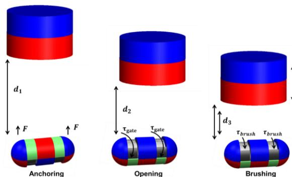
Figure 2. Operational flow: the EPM position triggers first the adhesion of the capsule to the intestinal walls, second the opening of the gates, and third the brushing of the mucosa.
