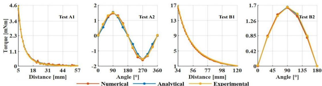
Figure 7. Torque curves obtained from tests A and B: comparison of experimental results, with the analytical and numerical models.
