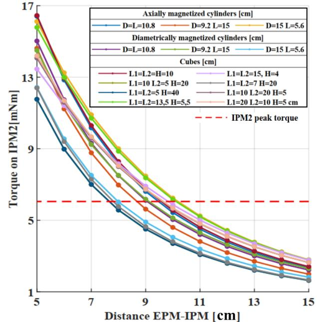
Figure 5. Torques induced on IPM<sub>2</sub> by different EPM with fixed volume of 1000 cm<sup>3</sup>, at variable distances IPM-EPM (results of the analytical model). The EPMs investigated are axially magnetized cylinders, diametrically magnetize cylinders, and cubes. The red line shows the peak torque for IPM<sub>2</sub>, which when reached, allow to rotate the magnet (brushing).
