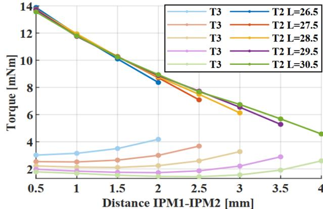
Figure 4. Peak torque curves of IPM<sub>2</sub> and IPM<sub>3</sub> varying the length of the capsule ( $L$  [mm]) and the distance between IPM<sub>1</sub> and IPM<sub>2</sub> (results of the analytical model). These values are those that need to be overcome by the EPM to open the gate ( $\tau_3$ ) and brush the mucosa ( $\tau_2$ ).
