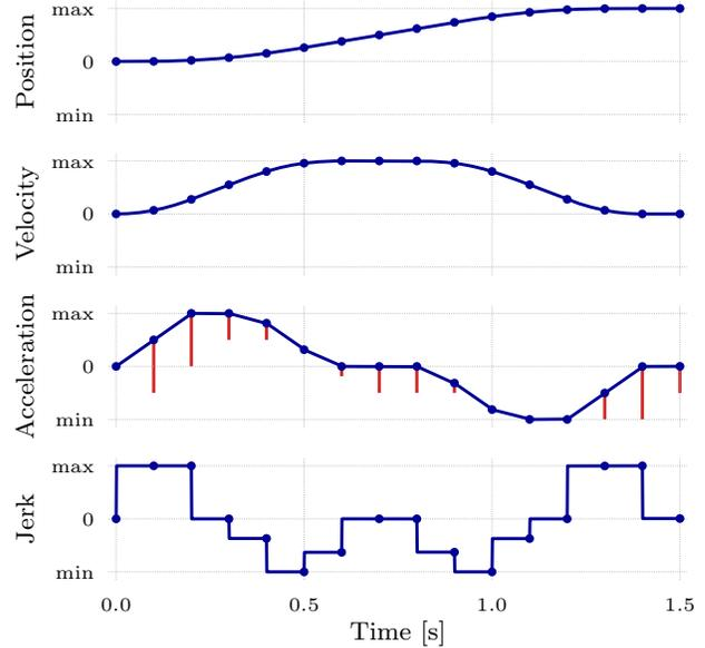
Fig. 1: Our method enables learning of robot trajectories that do not violate position, velocity, acceleration and jerk limits. At each decision step, a neural network predicts an action  $\in [-1, 1]$  that is linearly mapped along the range of safe accelerations (red line). Prediction frequency  $f_N$ : 10 Hz
