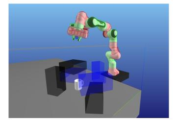
Fig. 6: Example experimental scenario for Franka Panda arm reaching through clutter to grasp a mug. The blue and black boxes are obstacles, and the green and red spheres on the arm represent the collisions for different robot links.
