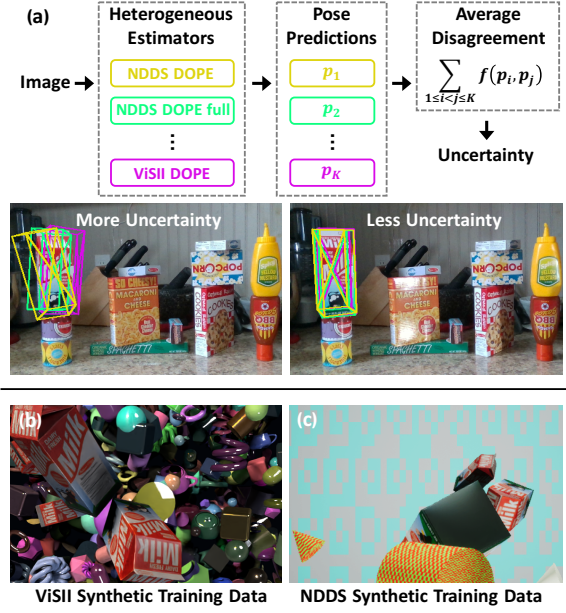
Fig. 1. (a) Illustration and examples of using an ensemble of heterogeneous models for uncertainty quantification. We calculate the average disagreement of K pose predictions from K different estimators as an estimation of uncertainty. The examples show the Milk object results of two images in the real-world HOPE dataset [1]. (b-c) Milk object examples in the synthetic ViSII (b) and NDDS (c) training datasets.
