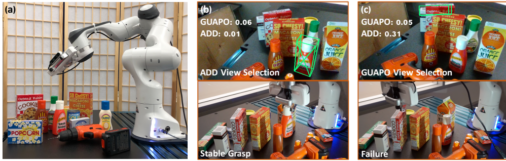
Fig. 3. (a) Experimental setup. (b-c) The view selection and grasping results of the Ketchup object from our method and GUAPO [17]. We use the NDDS DOPE model (green box) as the pose estimator and we quantify its uncertainty. For our method we use the average ADD disagreement between NDDS DOPE and NDDS DOPE full as the uncertainty. The numbers in (b-c) show the uncertainty quantification values of GUAPO and our method.
