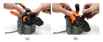
Fig. 8: Human intervention (when powered off): (a) manually close to grasp, (b) manually open.
