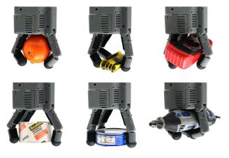
Fig. 6: The example grasps with different objects.
