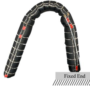
Figure 11. Eversion robot performing a  $146^\circ$  rotation, at 0.04 bar pressure in the main chamber.
