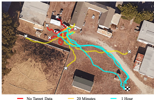
Fig. 6: Fast Adaptation to a New Environment: After training ViNG in one environment, we deploy the system in a novel environment, shown above. By practicing to reach self-proposed goals and using that experience to finetune the controller, ViNG is able to quickly gain competence at reaching distance goals in this new environment, using just 60 minutes of experience. Example rollouts towards a goal 35m away (marked by checkerboard circle) demonstrate ViNG self-improving from interactions in the barracks environment.
