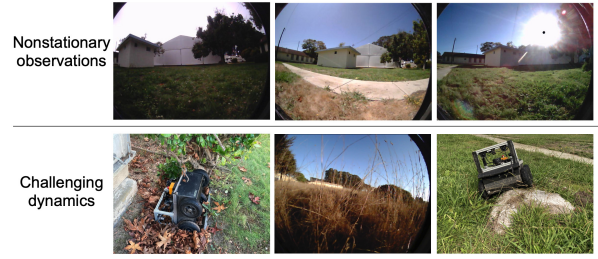
Fig. 2: Challenges with Real-World Navigation: (Top) Three observations taken from exactly the same position at different times of day exhibit large differences. (Bottom) While tall grass and inclined rocks are traversable, a hole filled with dry leaves is not. These examples highlight the challenges with geometric reasoning about traversability.
