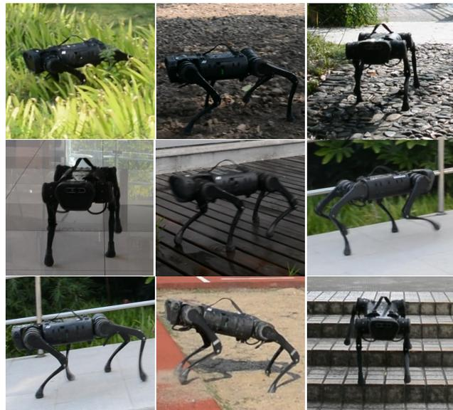
Fig. 1. Application of TERT on A1 robot over multiple challenging terrains.
