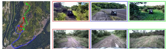
Fig. 5: Overview of large-scale navigation experiments. The leftmost figure shows a satellite view of the three courses: red, blue, and green. The top row shows sample aerial views of the courses, while the bottom row shows sample first-person robot images. The color of the rectangle around the picture denotes the course.
