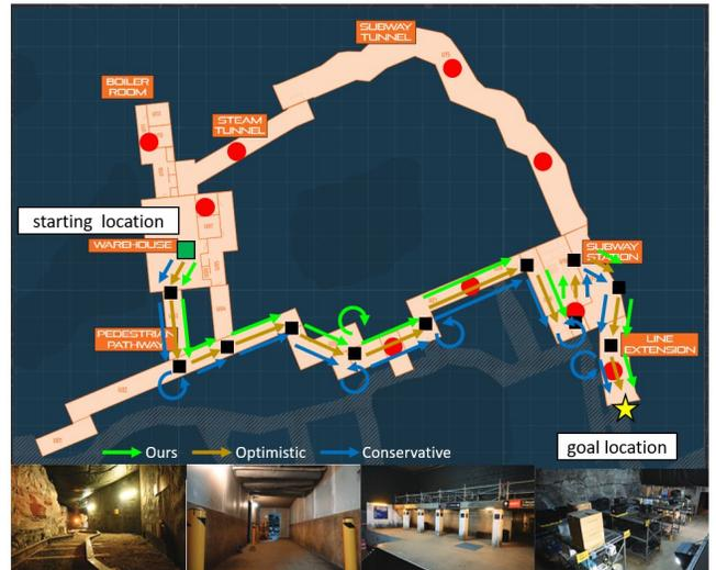
Fig. 4: Course map of the simulation based on real-world urban environment depicted by the photos on the bottom. Red dots on the map marked the location of stairs and rubble. The most likely paths computed by all the methods are overlaid on the map. The circular edges represent information gathering action.
