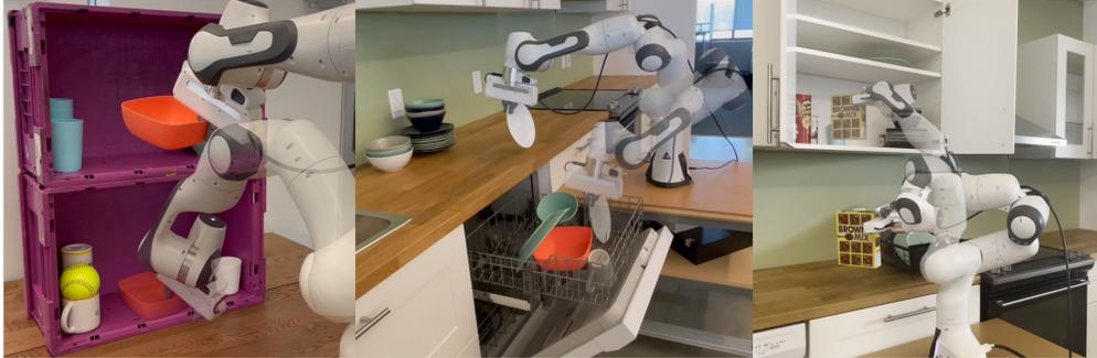
Figure 4: CabiNet is used for pick-and-place tasks in the real world. The scenes in the middle and the right are out-of-distribution environments in a real IKEA kitchen.
