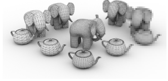
Fig. 3. Potentially Inconsistent Results (This image was produced by executing a variation of our sunflow benchmark — a real-world raytracing application detailed in Section VI — where the uniform block enclosing the image rendering is removed.)
