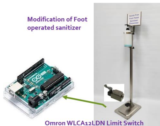
Figure 6.0. Modification of Foot pushing pedal sanitizer
