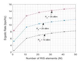
Fig. 3. Ergodic rate vs. Number of RIS elements (M) for different transmission power of BS  $(P_b)$
