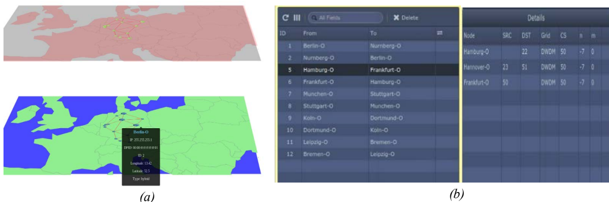
Figure 2. Julius user interface (a): emulated network topology overview, (b) manage established LSPs.
