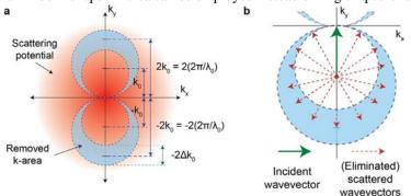
*Figure 1: (a) By inverse designing the scattering potential, (b) one can eliminate specific undesired scattered waves completely. The operational frequency can be easily tuned by varying the size of the targeted k-area.*
