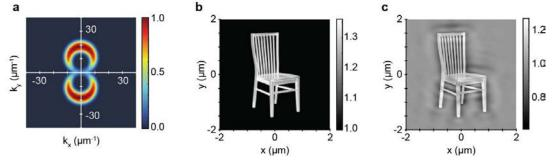
*Figure 2: (a) The area that is removed from the scattering potential is shown in wavevector domain. The spatial index distribution of the (b) original and the (c) modified object (exhibiting cloaking effect) is given.*
