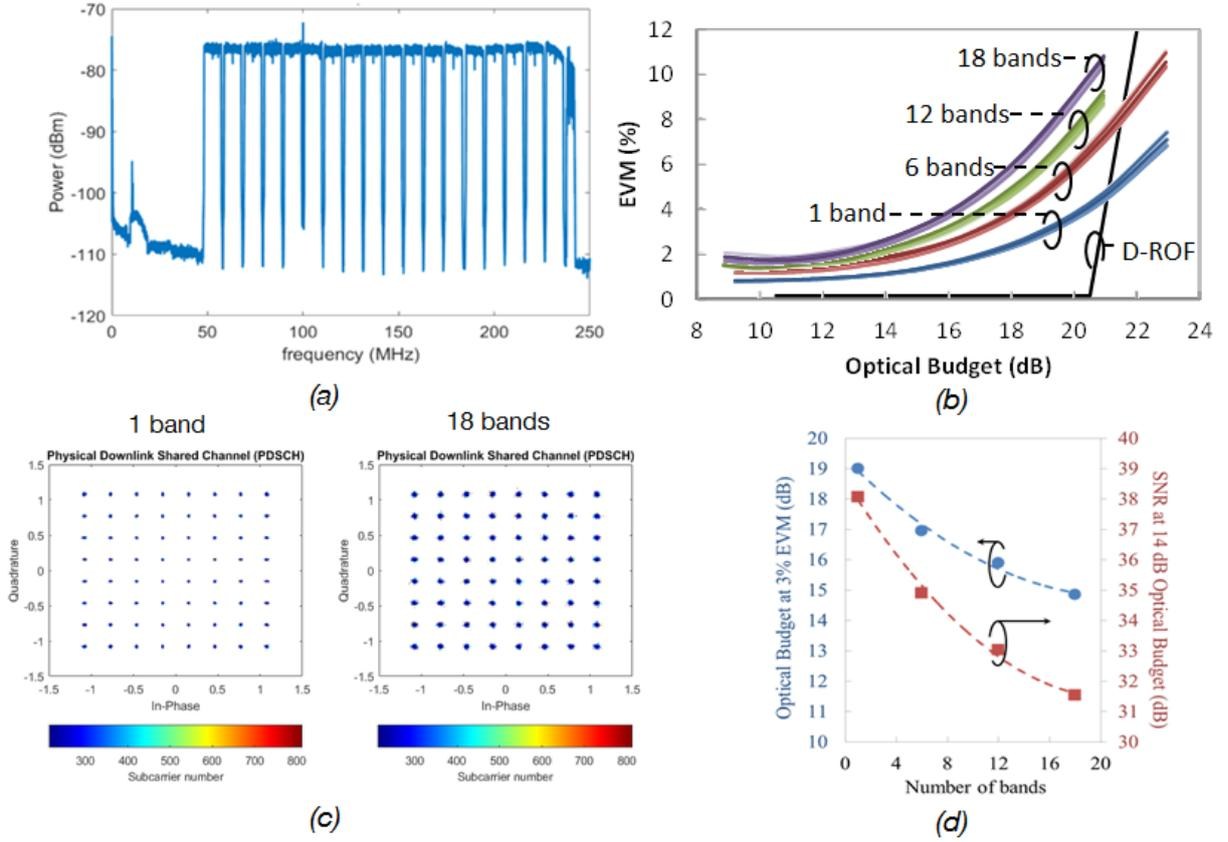
Fig. 3: (a) Received A-RoF spectrum. (b) EVM performances with received optical power. (c) Constellation diagram for 1 band and 18 bands transmission. (d) SNR and optical budget variation with the number of transmitted bands.
