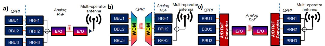
*Fig. 1: Distributed Antenna System architectures*
