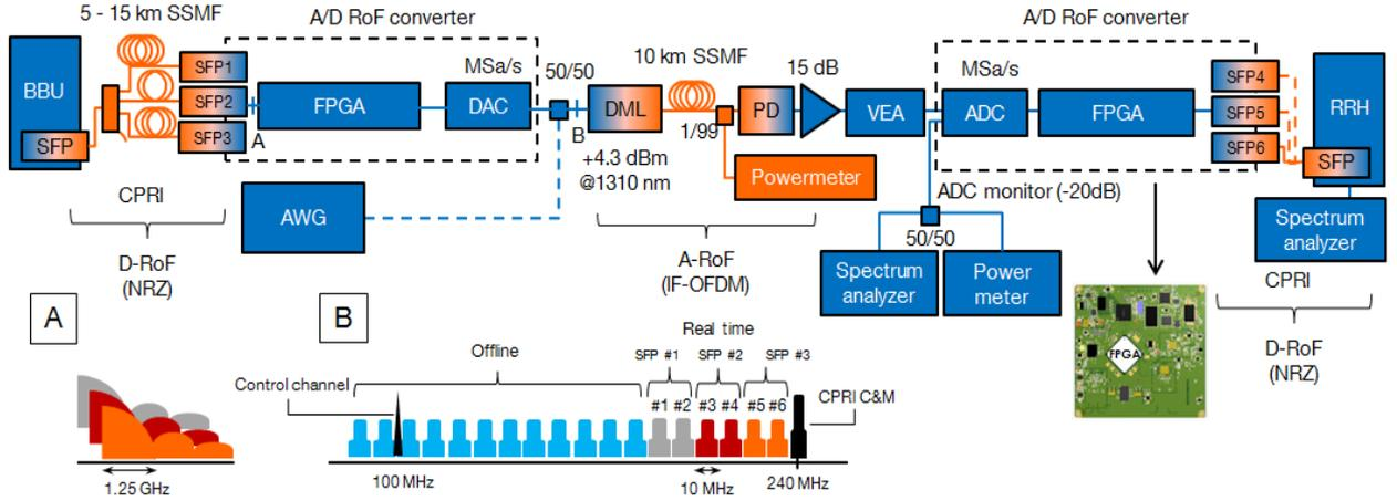
Fig. 2: Experimental setup
