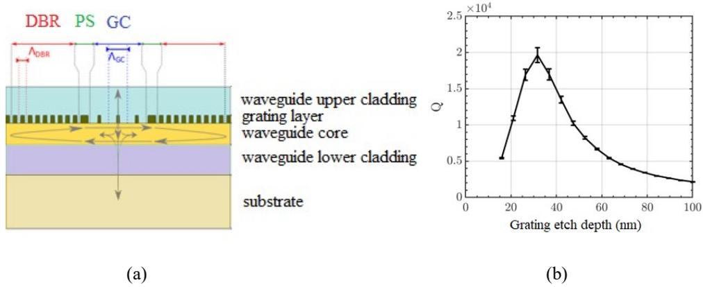
*Figure 1. (a) Schematic of conventional CRIGFs where the arrows indicate how the device operates. (b) Evolution of the  $Q$ -factor of a CRIGF as a function of the etch depth of the (DBR and GC) gratings*
