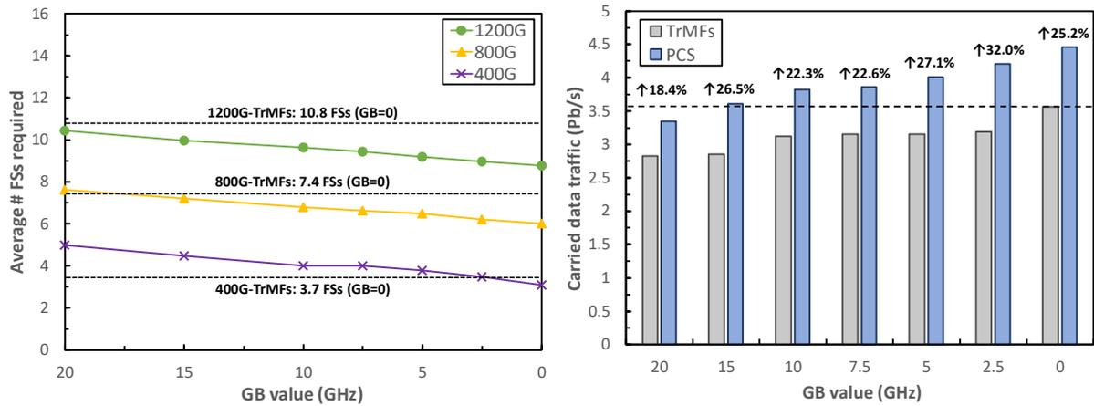
Figure 1. Average number of FSs required by a spectral super channel carrying a 400 Gb/s, 800 Gb/s and 1200 Gb/s demand using PCS, as a function of the GB value (left); total carried data traffic (in Pb/s) as a function of the GB value when using TrMFs or PCS (right).
