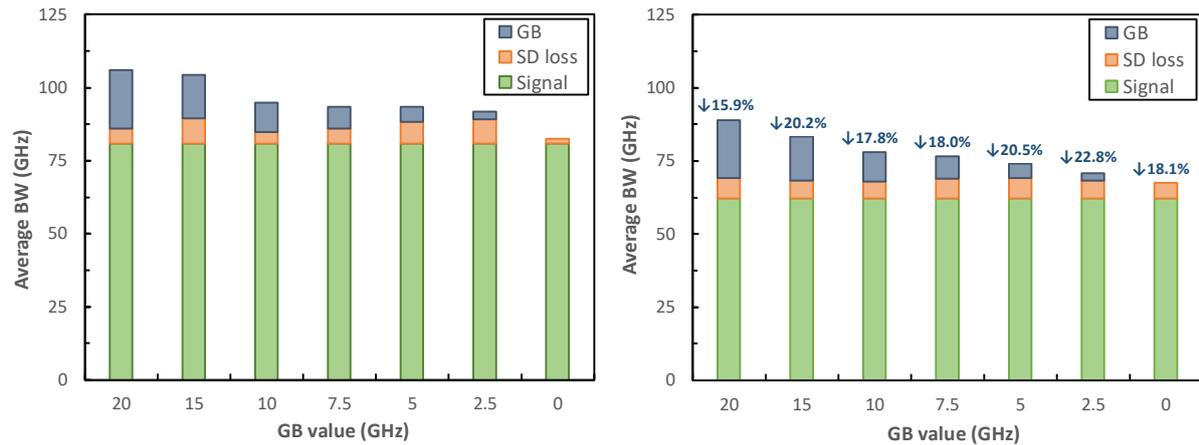
Figure 2. Average required BW by spectral super channels carrying the offered demands when using TrMFs (left) and PCS (right), both as a function of the GB value.
