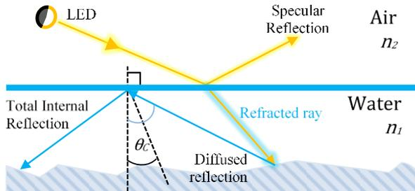
Fig. 2. Total internal reflection inside the water
