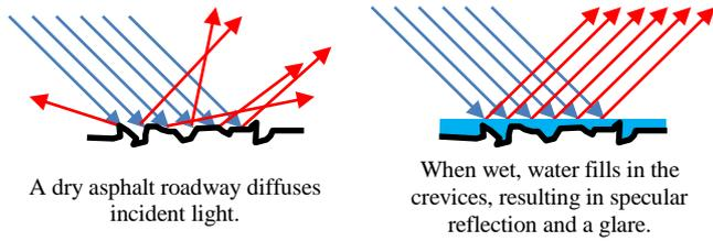
Fig. 1. Light reflection on dry asphalt roadway and wet asphalt roadway.
