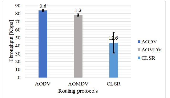
Figure 7: Network throughput based on the standard deviation.
