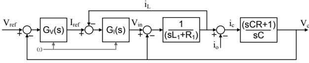
Fig. 3. Block diagram of the inner control loops.  $L_1$  is the inverter side inductance,  $C$  is the filter capacitance,  $R_1$  is the inverter side choke resistance and  $R$  is the damping resistance.
