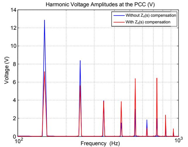
Fig. 9. Voltage harmonics at the PCC for the single phase rectifier with smoothing capacitor load ( $L_p = 84\mu H$ ,  $C_p = 235\mu F$  and  $R_p = 100\Omega$ ) with only inverter 1 connected to the microgrid.
