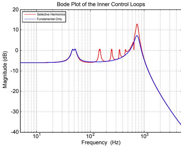
Fig. 4. Bode plot of the inner control loops with and without the selective harmonic control. The PR controller gains that were used in the simulations are:  $K_{pV} = 0.5$ ,  $K_{pI} = 2$ ,  $k_{iVh} = 200/h$ ,  $k_{iIh} = 200/h$ ,  $\omega_{cVh} = 0.001\omega_h$ ,  $\omega_{cIh} = 0.001\omega_h$  and  $h$  is the harmonic number. Hardware parameters for inverter 1 were considered for these plots as given in Table I.
