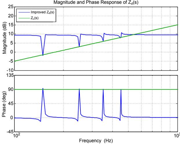
Fig. 8. Magnitude and phase response of the proposed virtual impedance transfer function  $Z_d(s)$  vs. the inductive grid side impedance  $Z_L(s)$  where  $R_V = k_{ph} = 3\Omega$ ,  $k_{ih} = |Z_L(\omega)|_{\omega=\omega_h}$ ,  $\omega_{ch} = \frac{0.02\omega_h}{h}$  and  $L_2 = 0.9mH$  is the grid side inductance.
