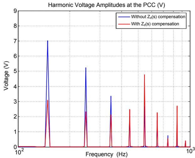
Fig. 10. Voltage harmonics at the PCC for the single phase rectifier with smoothing capacitor load ( $L_p = 84\mu H$ ,  $C_p = 235\mu F$  and  $R_p = 100\Omega$ ) when both inverters are connected to the microgrid.
