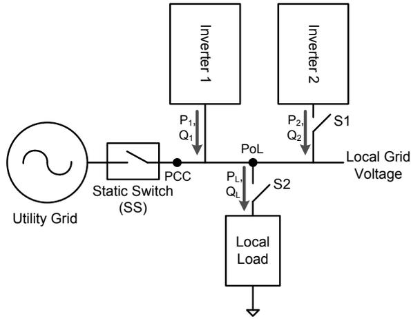
Fig. 1. Block diagram of the microgrid setup.
