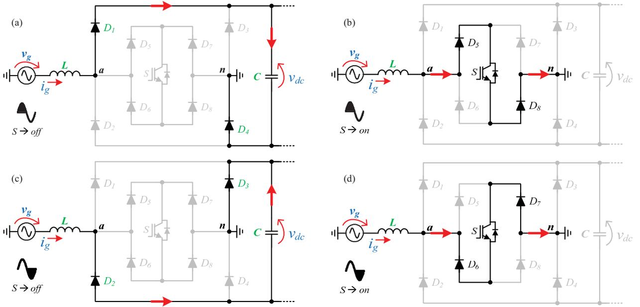
Fig. 2. Operation stages of the SSTL as active rectifier: (a)-(b) When  $v_g > 0$ ; (c)-(d) When  $v_g < 0$ .
