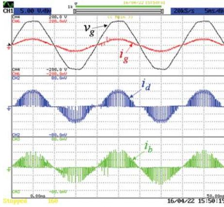
Fig. 9. Experimental results of the SSTL active rectifier: Power grid voltage ( $v_g$ : 50 V/div); grid current ( $i_g$ : 5 A/div); Current in the diode bridge ( $i_d$ : 2 A/div); Current in the bidirectional cell ( $i_b$ : 2 A/div).
