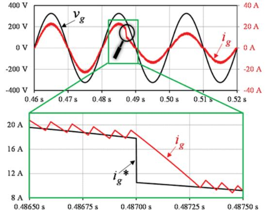
Fig. 4. Simulation results of the SSTL active rectifier during a transient variation in the power from 3.6 kW to 3 kW: Power grid voltage ( $v_g$ ); Grid current ( $i_g$ ); Grid current reference ( $i_g^*$ ).
