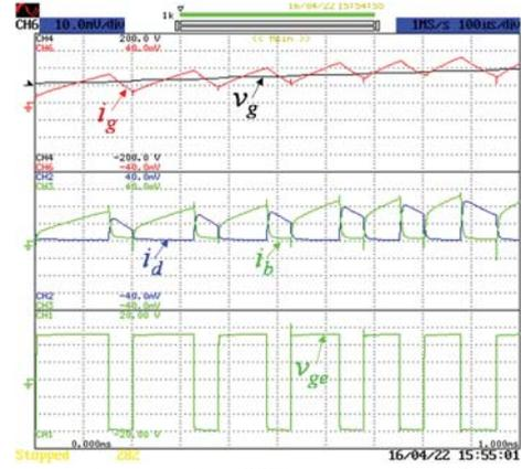
Fig. 10. Experimental results of the SSTL active rectifier: Power grid voltage ( $v_g$ : 50 V/div); grid current ( $i_g$ : 1 A/div); Current in the diode bridge ( $i_d$ : 1 A/div); Current in the bidirectional cell ( $i_b$ : 1 A/div); Gate-emitter voltage of the IGBT ( $v_{ge}$ : 15 V/div).
