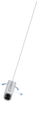
Fig. 6. Yaw with translational motion experiment
