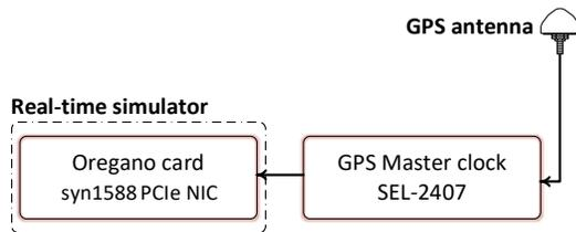
Figure 6. Synchronization of the real-time simulator with Oregono syn1588 PCIe NIC board and GPS master clock SEL-2407.
