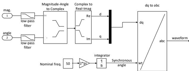
Figure 4. Implementation of phasor-to-waveform conversion.
