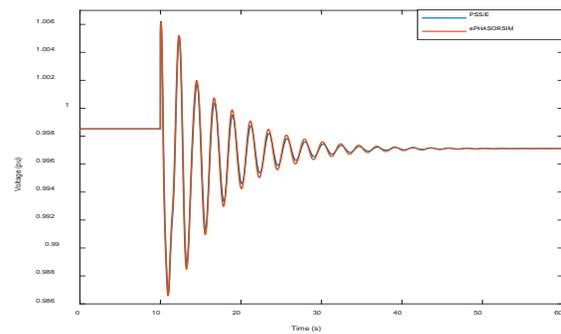
Figure 7. Voltage at bus 7 obtained from PSS/E and ePHASORSIM simulations when a line between bus 7 and 32 is tripped.
