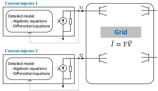
Figure 1. Illustration of power system dynamics simulation.
