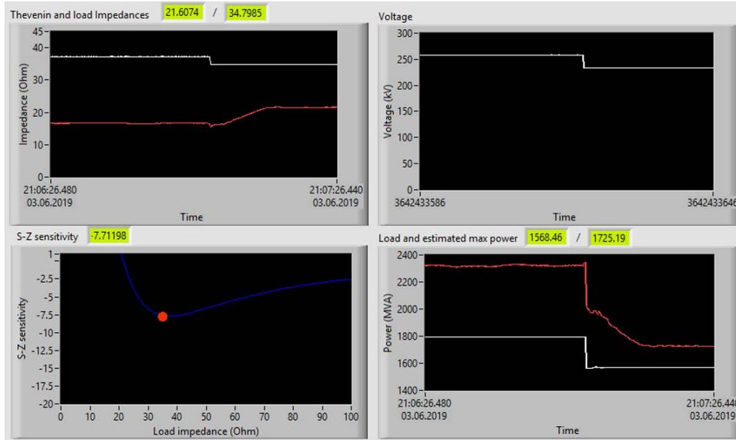
Figure 10. The online voltage stability monitoring application detects that the load at node 25 is close to voltage stability limit.
