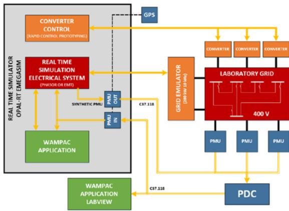
Figure 2. Overview of the testing platform.
