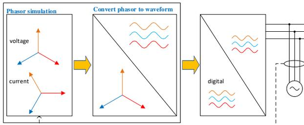
Figure 3. Conversion of phasors to waveforms to enable PHIL testing.
