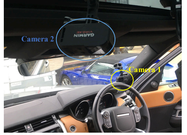
Fig. 4. Cameras inside the vehicle. Locations have been highlighted by different colours.
