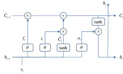
Fig. 2: The structure of the LSTM.
