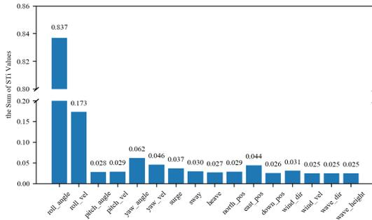
Fig. 4: The statistical result of sensitivity analysis for the one-step model.
