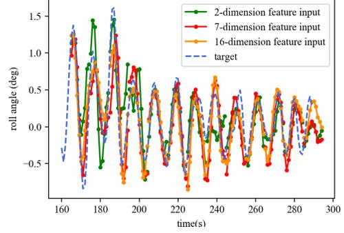
Fig. 9: The result of the ten-step ship model prediction.
