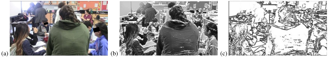
Fig. 3: AM-FM representation for classroom environment. (a) Classroom image. (b) AM component. (c) FM component
