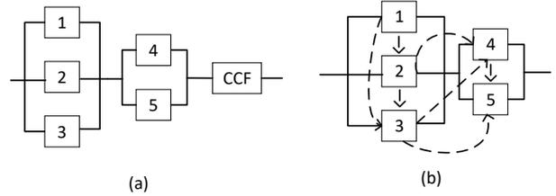
Fig. 2. System structures with CCFs and cascading failures
