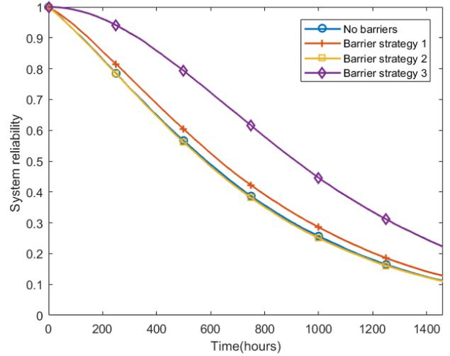
Fig. 4. The effects of safety barrier B<sub>4s</sub> for cascading failures
