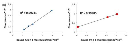
**Fig. 3.** Fluorescence versus spotting concentration compared to fluorescence (a) versus serum bound to spot label-free measurement (b). Results show that CaFE platform yields calibrated, linear responses for allergy testing analysis compared to traditional "semi-quantifiable" analysis. For the CaFE measurement of Ph1 Timothy grass allergen, the last point was removed from the calibration due to saturation of bound serum.
