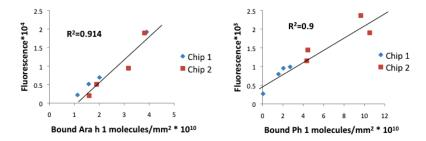
**Fig. 4.** Fluorescence signal of labeled IgE versus bound target to spot label-free measurement to investigate calibrating chip-to-chip variability for peanut (left) and timothy grass (right) allergens. Results show that CaFE platform yields calibrated, linear responses despite chip-to-chip for a variety.
