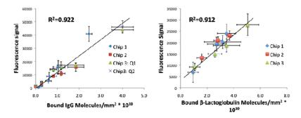
Fig. 2. Fluorescence versus bound target to spot label-free measurement for rabbit IgG (left) amd B-lactoglobulin(right). For IgG calibration of Chip 3, Q1 and Q2 analyze spot to spot variability. Results show that CaFE platform yields calibrated, linear responses from chipto-chip for a variety of proteins.
