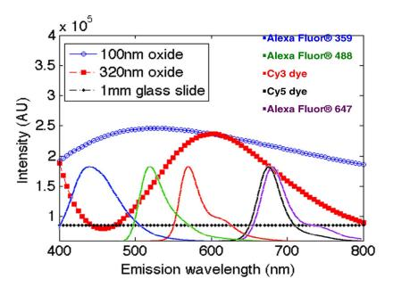
Fig. 1. Fluorescence intensity values for  ${\rm SiO_2}$  thicknesses of 100nm and 320nm compared to a microscope slide. Over all wavelengths, 100nm oxide has more than 2-fold emission enhancement compared to glass for a broad range of fluorophores. To compare, 320nm oxide enhances Cy3 and Cy5 emitters about 1.9 times compared to glass.
